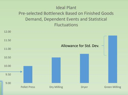
The Maximum Deviation of a preceding process sets the starting point of the subsequent operations
