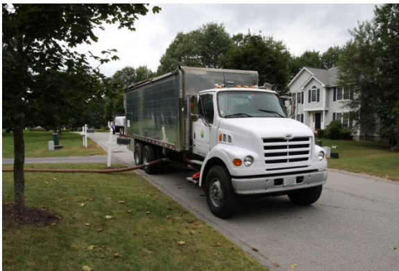
A bulk delivery truck equipped with pneumatic hosing...
