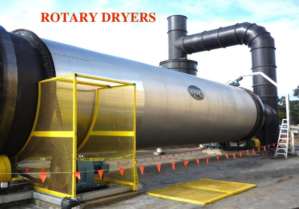
"Rotary Dryers shall have automatic spark detection and extinguishing systems installed between the dryer drum and downstream material handling equipment, such as cyclones or wind boxes."
