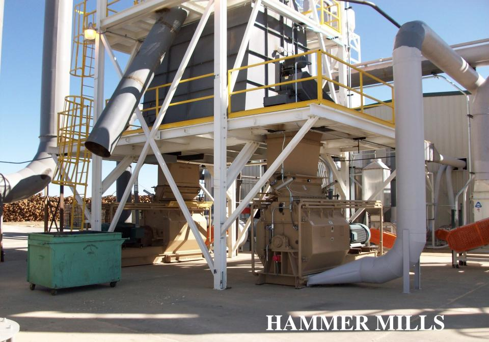
"Unless the particulate size reduction equipment is strictly dedicated to handling green material or is pressurized with steam, it shall be considered a highfrequency ignition source."
