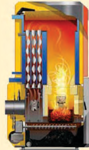
Wood chip boiler
