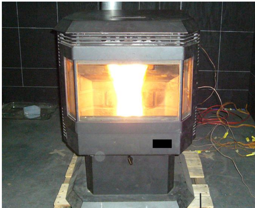
Figure 3. Top-feed pellet stove undergoing testing.
