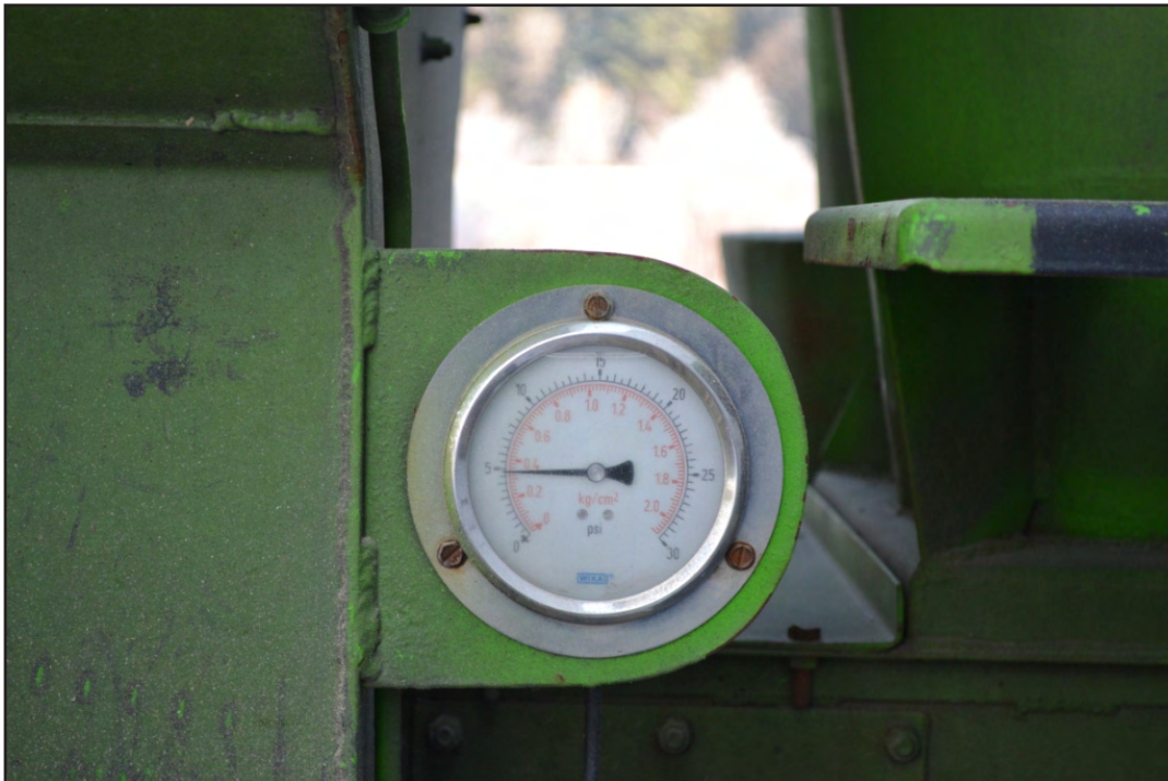
Figure 4: Delivery hose pressure gauge
