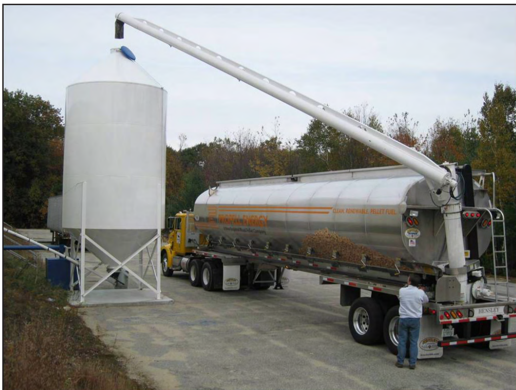
Figure 2: Auger truck delivering to an outdoor silo
